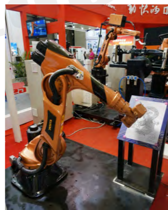
Robot's drawing application based upon the off-line programming
